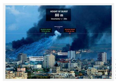
The height of burst of the M825 WP projectile is established by using urban structures as reference measures.
